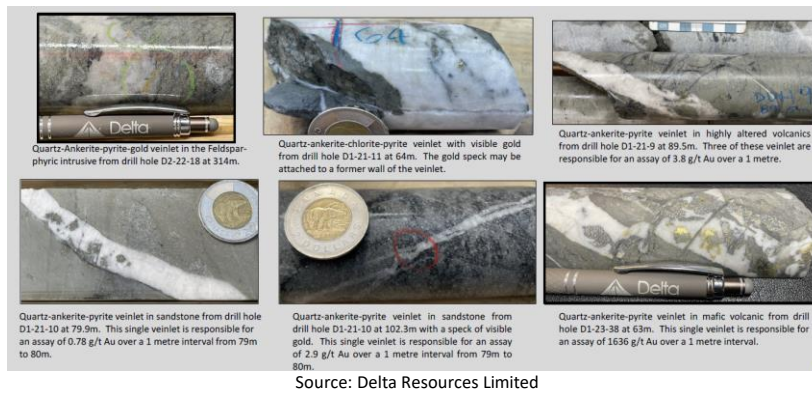
Figure 3. Eureka gold deposit mineralization including samples with visible gold.
